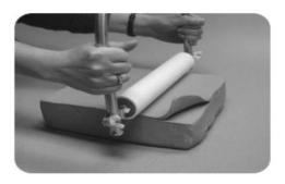
The rolling pin is helpful for the rolling of thick layered clay. The wooden slat is the tool over which the clay is placed, and the pin rolling is performed.
