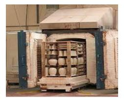
For firing of the clay, a kiln is employed. It is a type of furnace which is made up of refractory materials. They work with the help of electricity, fuel, gas, coal, wood, etc.
