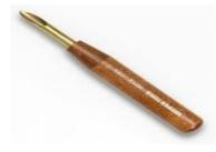
For the trimming of piercing clay in the ceramic, hard pointed wire is fixed at the head of the handle.
